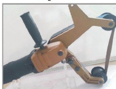
Tensioner arm for replacing the sanding belt
