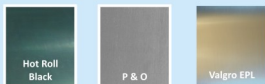
Figure: The photographs above are of three different surface treatments applied to hot rolled strip (L to R: Hot Roll Black, Pickled & Oiled and Valgro EPMS)
